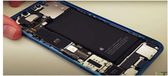
Figure 6 Battery of iPhone 13 pro [17].
