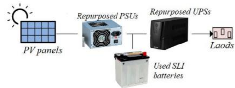
Fig 2. Solar PV system containing second life components [11]
